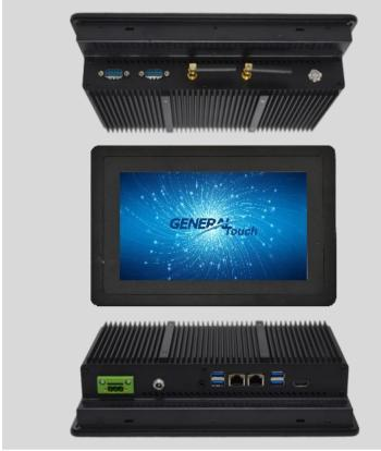
The General Touch's industrial panel PC series is the result of leveraging years of experience in building AiOs and serving the Industrial clientele. Being mindful of the varying industrial environments, the Touch Panel PC features panel mount & VESA mount installations, fanless heat dissipation, front sealing that meets IP65 rating and an aluminum alloy frame for durability. The operating temperature ranges from -15°C to 60°C.
