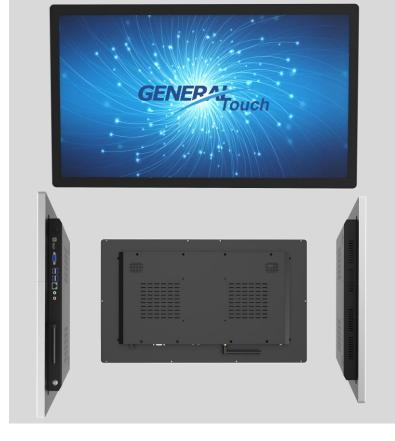
General Touch's breed of Closed Frame Touch computer is characterized by its unified design with AL Alloy frame edges. This sleek and sturdy contraption is loaded with enticing features and options that cater to different requirements including operating on Android, Windows and Linux platforms. The Android version is equipped with a Rockchip processor, while the Windows and Linux versions utilize powerful Intel processors.
