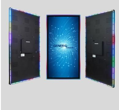
The LED-Framed monitor dazzles with ambient lighting effects on the front and/or back of its sides. The color, style, and rhythm of the lights can be used as adornments, alerts, attractions, flags, indicators or fanfare that will surely boost the interactive functions of a display for both the users and operators.
