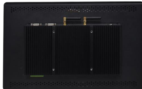
Slanted Rear Side of the Industrial Panel PC
