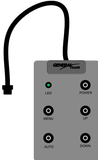
Fig 12 OSD Remote Diagram
